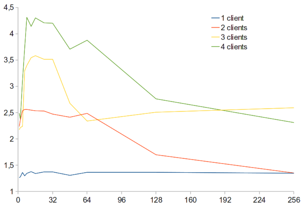
Figure 6.3: FPS for different numbers clients with different segment sizes.
